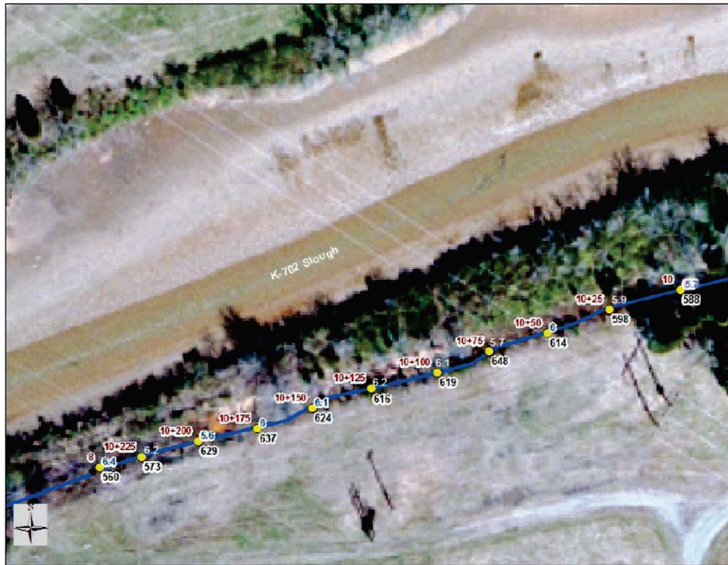
Fig. 3.21. pH and conductivity profile for coal ash sluice channel—April 2011.
